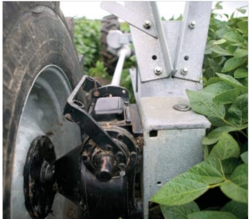
Zimmatic's tow/non-tow final-drive gearbox uses a bale engagement lever to disengage the gearbox for towing. When you're ready to irrigate, simply re-engage the gearbox with the lever.
